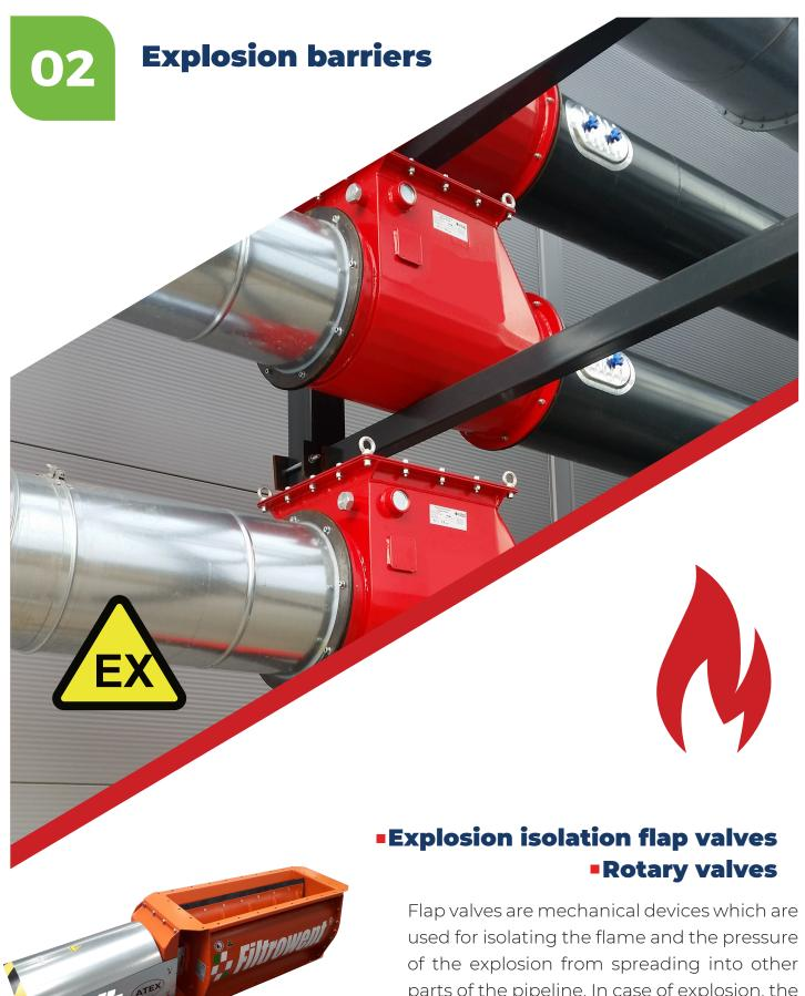
Flap valves are mechanical devices which are used for isolating the flame and the pressure of the explosion from spreading into other parts of the pipeline. In case of explosion, the flap valve is closed by the shock wave and this way prevents the explosion from spreading. The flaps are installed on pipelines at a specified distance, thanks to which they work as a multilevel protection of a dedusting system.
