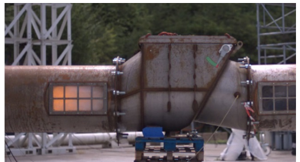
Photos taken during testing of VIGIFLAP d800 mm (protected vessel of 10m 3 , dust Kst250 bar.m/s)
